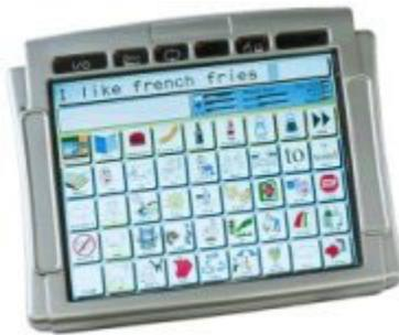
The Vantage is an augmentative communication aid that uses the Minspeak language system for storage and retrieval of messages. It is designed to be used by anyone who, for whatever reason, has difficulty speaking and could benefit from an AAC system.
