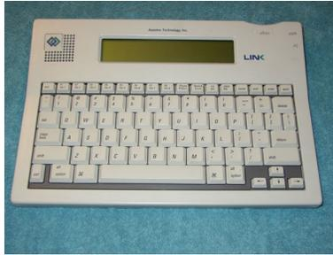
The Link is a talking word processor. You can use it to write stories or reports, take notes, and more. Files are easily transferred to a computer with the appropriate cable. You can also print directly from the device.
